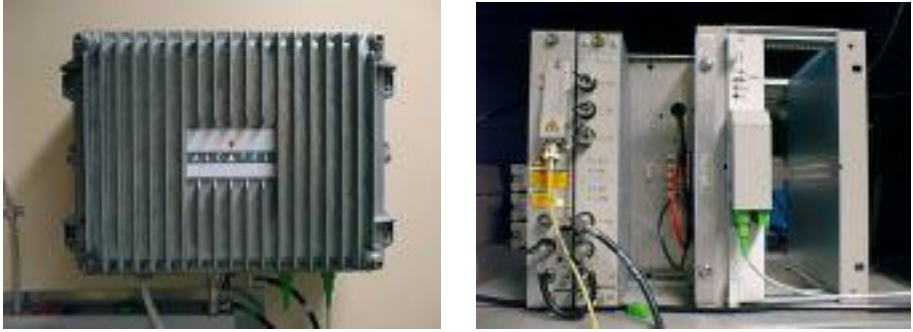
Fig. 7. Headend and BONT Optical Components
